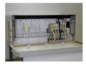
The set of control computer with communication unit WTB 2000 and local I/O modules of CZ-CAN series.
