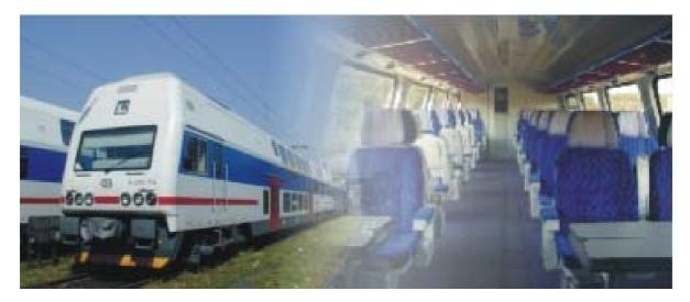
**EMJ 471** is a suburban double-decker for the lines with voltage 3 kV DC. Design speed of the train unit is 160km/h. The train unit is designed for climatic conditions  $-30^{\circ}$ C .. +40°C. It consists of three coaches, each of which is intended for passengers, but has different equipment.
