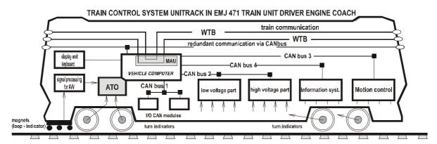
The system performs control, communication, diagnostic and filing functions. The system includes a database of timetables and relevant software, which enables to monitor relevant observance of or deviations from the train traffic diagram. The driver's stand is equipped with a keyboard and graphic display unit with touch screen, which displays all data including that of the speed controller and ATO – Automatic Train Management.
