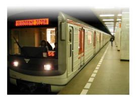
These reconstructed vehicles have been equipped with modern communication and control systems, which were developed and manufactured by UniControls to fully meet European standards. Data communication in the train is a backbone of the whole control, information and diagnostic system. The communication system is based on IEC 61375-1 standard TCN – Train Communication Network. The standard defines two communication buses, in particular WTB and MVB
